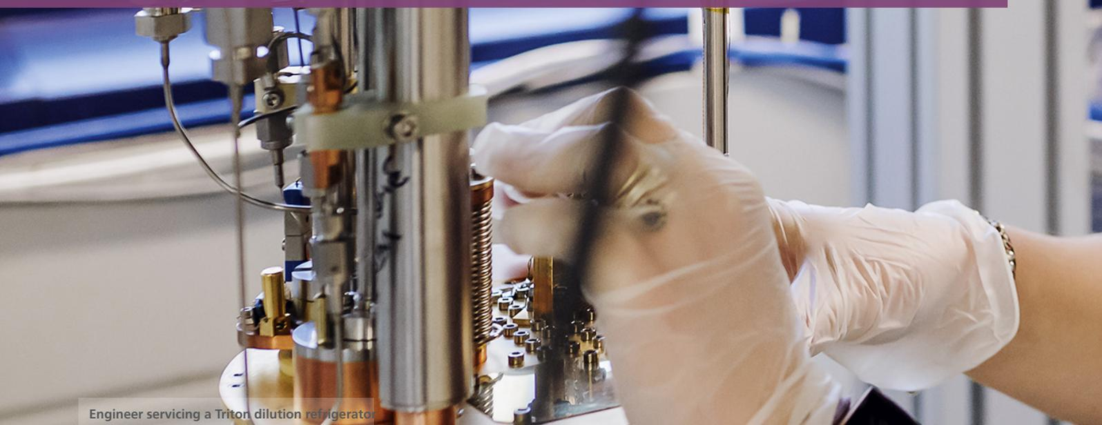
Engineer servicing a Triton dilution refrigerator
